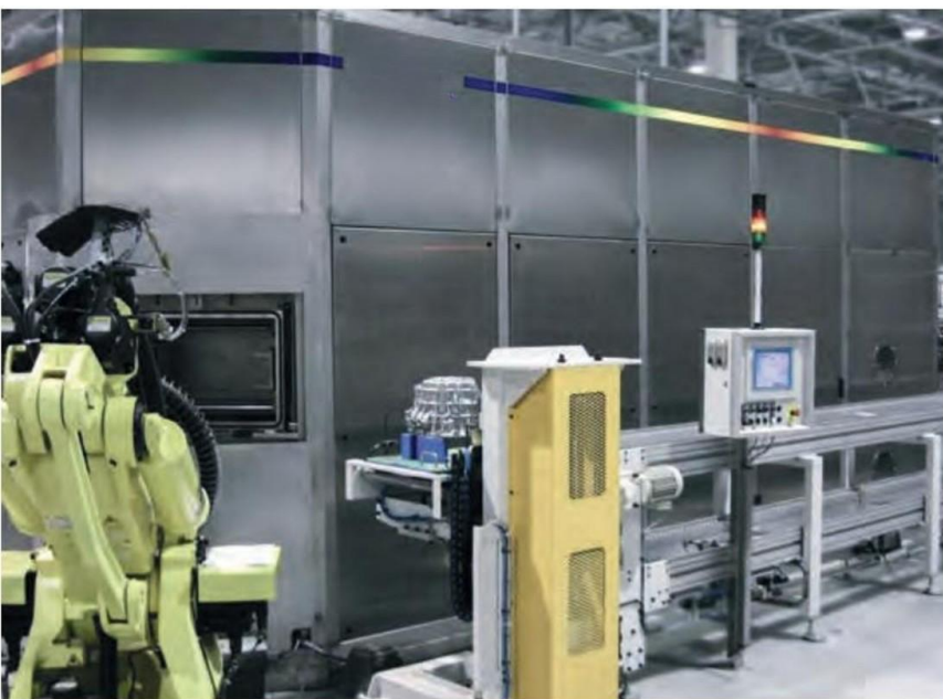
RT - Rotary transfer machine for cleaning gear units
